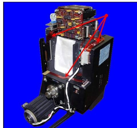
A-M CPT's new flexible circuit harness, shown wrapped around a TOW-2 optics chassis, precisely fits its host and provides many benefits to the Army over legacy models.
